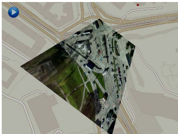
A screenshot from the new ProjectedVideo SDK sample, showing a projected video stream playing on top of OpenStreetMap vector data..
