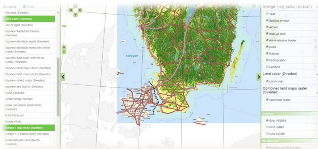
Figure 4. Screen shot of the Carmenta Web Explorer GUI with the Catalogue Panel to the left and Layer Panel and utility layer controls to the right.
