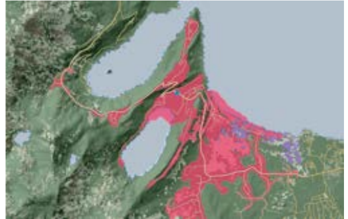
Figure 17: An isochrone map generated from a network consisting of roads and terrain for a vehicle with real-time speed. The isochrone is generated from the blue circle as reference point. The isochrone is generated from a road as initial point.
