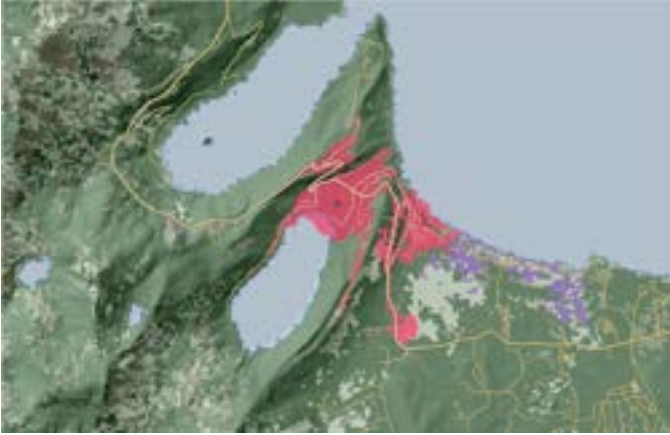
Figure 18: An isochrone map generated from a network consisting of roads and terrain for a vehicle with real-time speed. The isochrone is generated from the blue circle as reference point. This figure is similar to figure 17 yet the isochrone area is much smaller due to the starting position being on terrain. Terrain has a lower vehicle speed.
