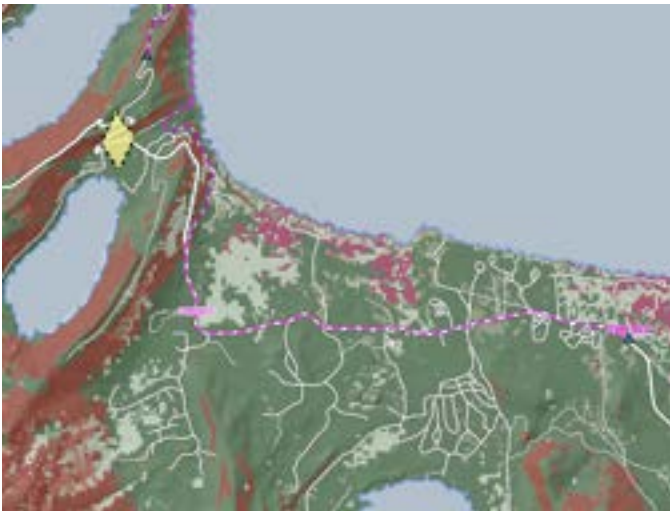
Figure 7: Based on the scenario depicted in figure 3 the shortest path solution from figure 4 will change if an obstacle appears along the original planned route. An obstacle area painted in yellow has been placed in the first traffic situation just below the starting position. The new solution, painted in purple dashed lines, circumvents this obstacle by going along the shore. The new travel time is 23 minutes and 46 seconds. Using equation 2 the penalty time is 14 minutes and 2 seconds.
