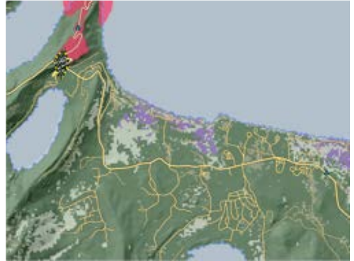
Figure 8: Based on the solution presented in 6. When applying the same obstacle from figure 7, the isochrone area painted in red has decreased in size drastically from figure 6. Using the 11-minute travel time constraint, the starting position and the destination is no longer contained inside the red area. The dramatic shrinking of isochrone area is due to the large penalty time added from applying the obstacle, which is observed in figure 7.
