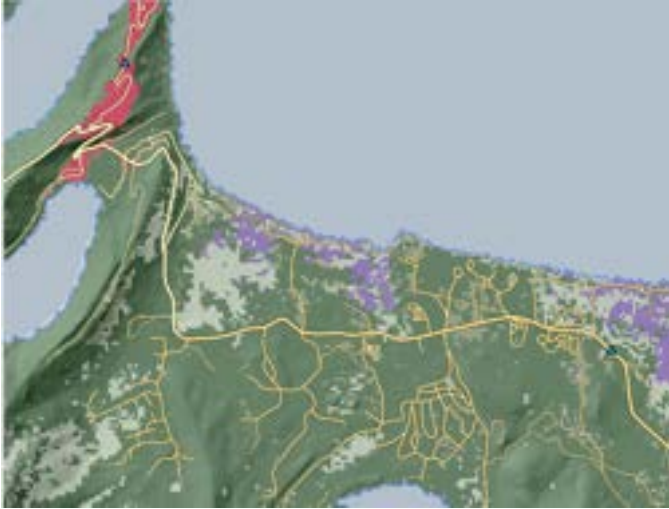
Figure 5: Studying the shortest path problem using the shortest path tree visualized using isochrones. The conditions of this scenario is presented in figure 3. The isochrone is calculated using the top left starting position as the reference vertex and the solution is visualized as a red area. The red area visualizes all the positions reachable within the travel time constraint put on the isochrone. In this case the travel time constraint is 3 minutes.
