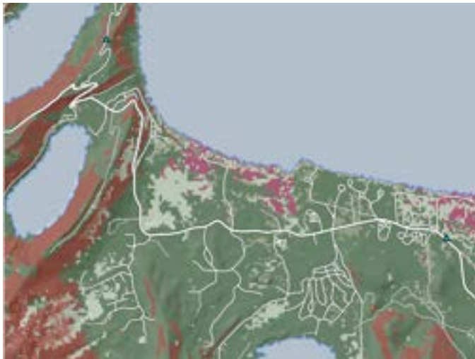
Figure 3: A compact routing scenario using a mixed network of roads and traversable terrain together with a proposed vehicle. Traversable terrain is painted green while non-traversable is painted red. Roads are visualized using white lines with thickness illustrating road type class.
