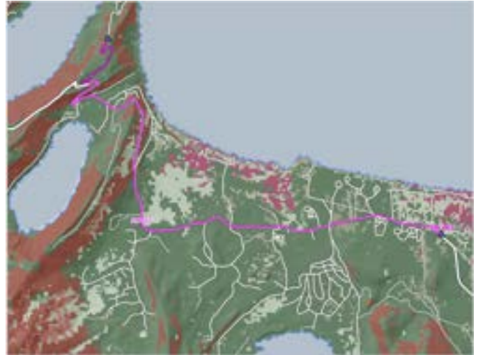
Figure 4: A solution to the quickest path problem using the scenario described in figure 3. Solution was found using the D*-algorithm. The purple line visualizes the route and the travel time is printed in text along the route. The travel time is 9 minutes and 44 seconds.
